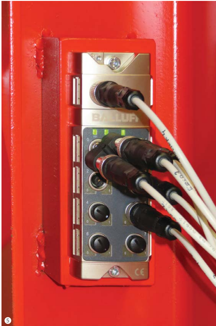
Figure 5: HUB connections of all the solenoid valves and sensors of the system.
