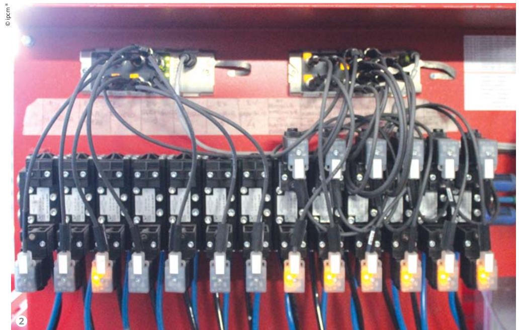
Figure 2: Electric circuits equipped with an inverter to allow the selection of the abrasive throw speed.
