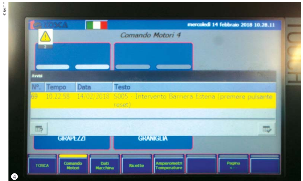
Figure 4: The touch screen operator panel for setting all the shot blasting machine's functions.
