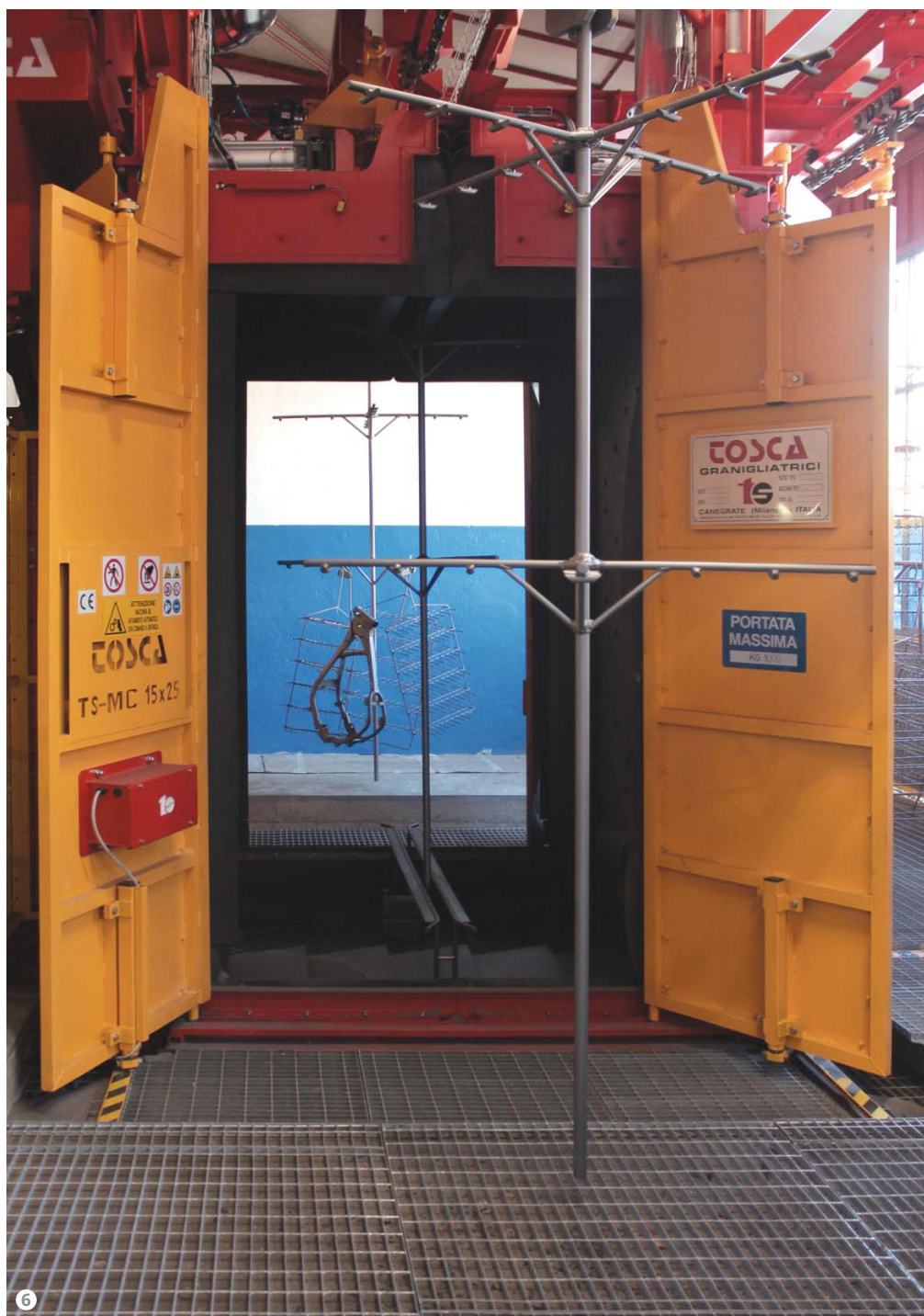
Figure 6: The shot blasting machine is equipped with two automatic doors operated by pneumatic cylinders.
