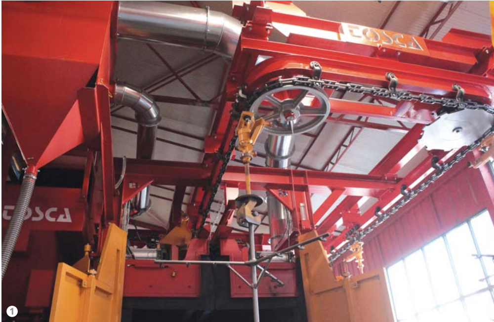
Figure 1: A detail of the ring-shaped one-rail conveyor, which enables to load and unload parts on different hooks outside the chamber while another one is being subjected to shot blasting.
